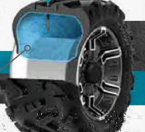
Once a leak occurs, the tire sealant rushes out of the tire and quickly creates a permanent solid plug.
