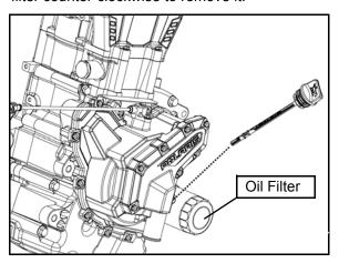
10. Using a clean dry cloth, clean filter sealing surface on the crankcase.
