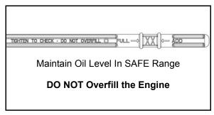
NOTE: A rising oil level between checks in cool weather driving can indicate contaminants such as gas or moisture collecting in the crankcase. If the oil level is over the full mark, change the oil immediately.
