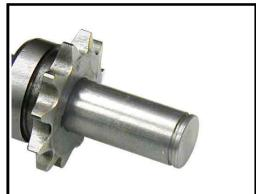
Steering shaft and sprocket
