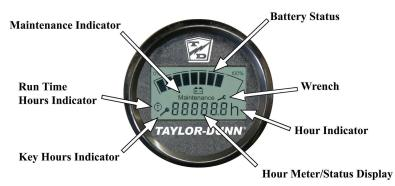
The Smart View Display (SVD) functions as a Battery Status Indicator (BSI), Hour Meter (HM), speed controller status monitor, and as an optional maintenance monitor feature. The operation of each of these functions is listed below.
