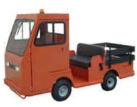
B2-48 with Steel Cab, Foldaway 4-Passenger Seat an
