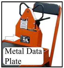
The vehicle data plate will be in one of two locations depending on type of data plate and manufacturing date
