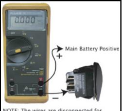
NOTE: The wires are disconnected for reference only. The test must be done with the wires connected to the switch.
