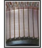
Properly undercut and cleaned commutator segments
