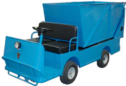
B 2-48-36 Equipped with optional hydraulic dump bed
