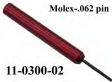
Molex # 11-300-02: Pin Removing Tool Removes 0.062 diameter pins from Molex rectangular harness connectors. Not available from Taylor-Dunn. Purchase from any local electronics distributor.
